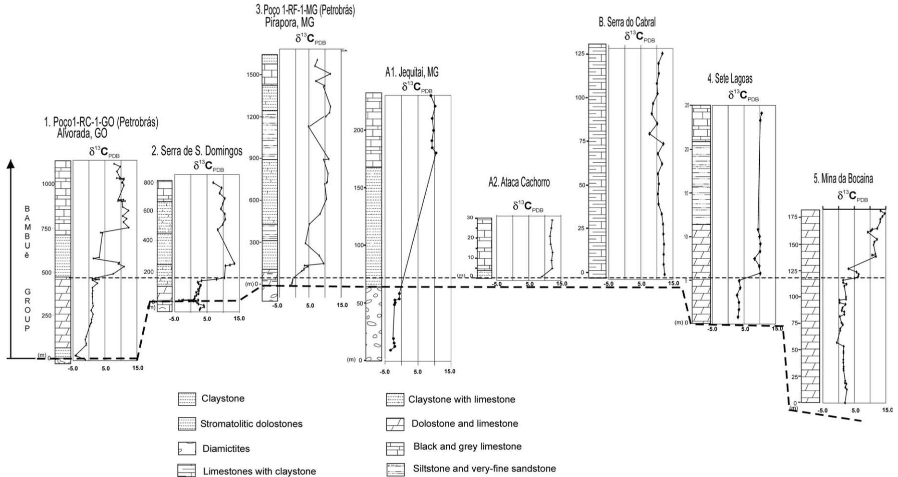
Fig. 4. Carbon isotope variations of the Bambuí Group with the representation of the positive  $\delta^{13}C_{PDB}$  excursion mark. 1, Alvorada (1-RC-GO) log according to Martins (1999); 2, Serra de São Domingos log according to Santos et al. (2000); 3, Pirapora (1-RF-1-MG) log according to Chang (1997); 4, Sete Lagoas log according to Santos et al. (2000); 5, Mina da Bocaina log according to Martins (1999); A1, A2 and B this paper. Locations of the logs are shown in Fig. 1.
